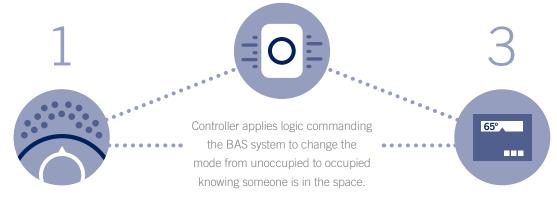
Occupancy sensor detects a presence in the boardroom when the room is known to be in unoccupied mode.
